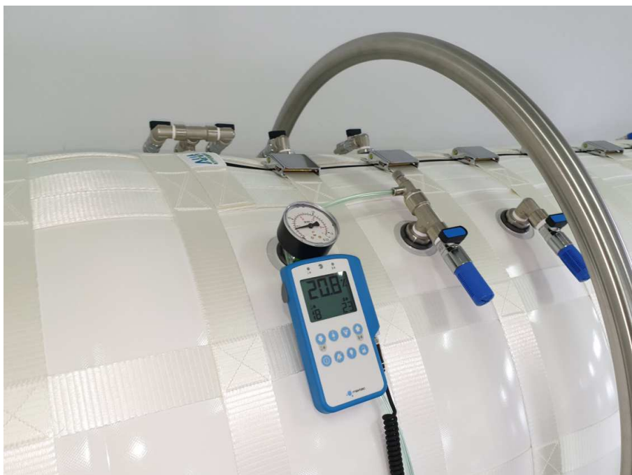
Oxygen monitoring analyser with alarm
